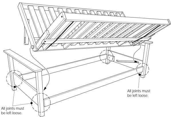
Insert the decks into the partially completed frame. This is where a helper may be useful.
