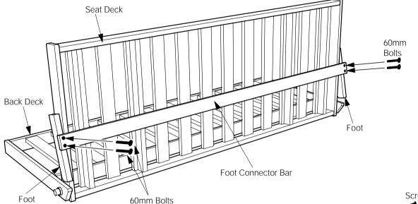
Lift the Seat Deck so it resting on the Back Deck. The feet should be pointing downwards.
